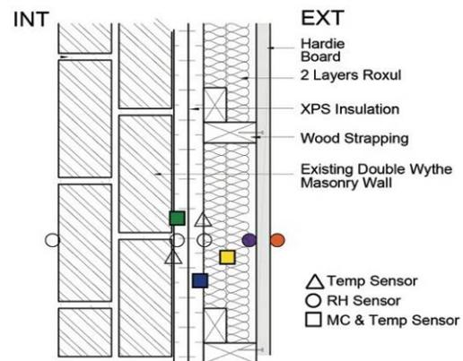
Fig 5: Sensors locations used in full scale retrofit at 111 Russett Avenue
