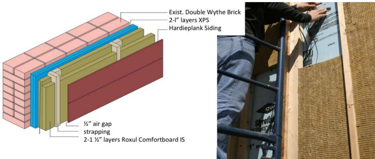
Fig 6: The image on the left indicates the exterior retrofit assembly chosen to be installed on the full scale field study with embedded sensors (right).
