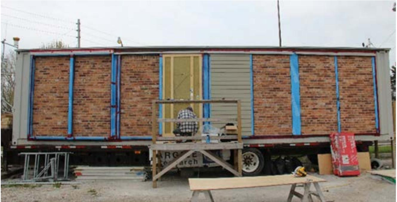
Fig 3: Test walls in Natural Exposure Test Hut
