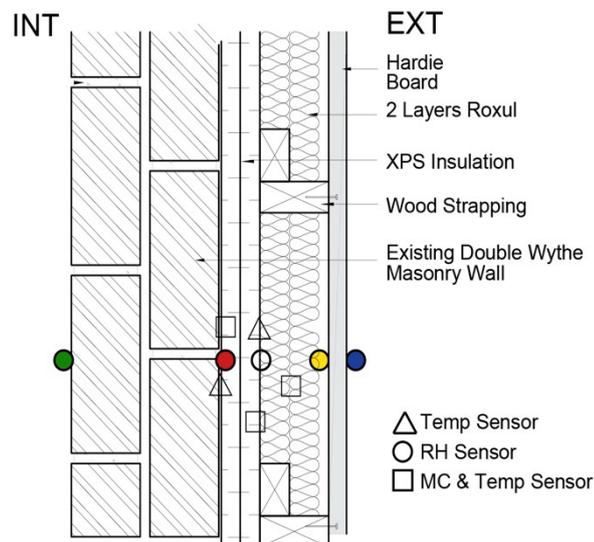
Fig 3: Sensor Diagram for Exterior Retrofit Wall 06 Test Hut
