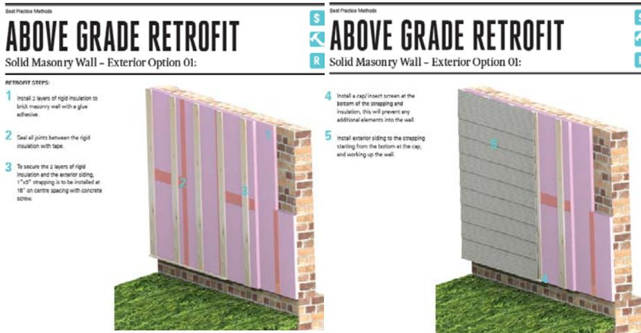
Fig 6: Excerpt from Chapter 4 showing Step-by-Step Installation. The top right corner outlines the criteria that this solution best meets, like cost, constructability and thermal resistance (efficiency)
