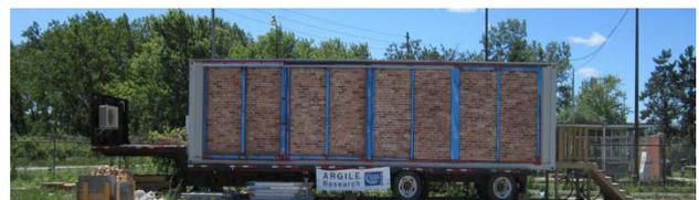
Fig 7: Exterior view of ARGILE's Test Hut in Toronto, testing 8 wall compilations for the guide
